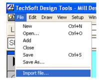
A pop up menu will appear from which you must chose the file location. The type of file that we require is a .DXF file. Select the drop down arrow to the right of the box for File of type: This will produce a drop down menu from which you can select DXF Files. Find the file named Flat pattern - Base.dxf and select Open.
